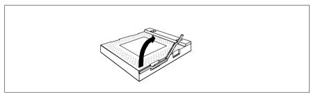
Figure 8: Opening the socket lever
